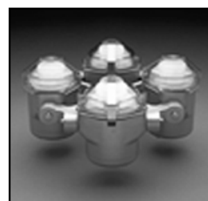
5800216 Economical Rotor includes four Forma 5800316 Buckets with clip-on domes.* 4 x 750 ml to 3400 RPM/2550 xg
