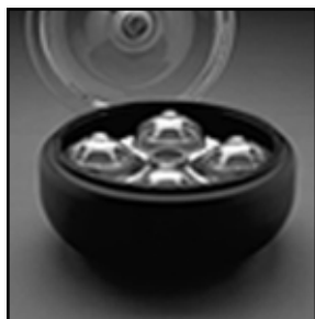
5800218 High Speed Sealed Rotor includes transparent sealed windshield lid and four Forma 5803218 Sealed Buckets.* 4 x 750ml - to 4600 RPM/4550 xg
